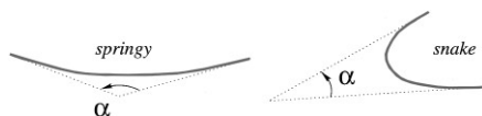
FIG. 11. Definition of the exterior angle \alpha , measured between the ends of a flexible fibre.
